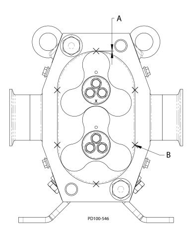
Figure 64 - Radial Clearance Check
