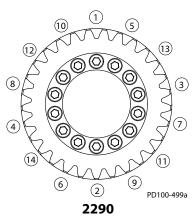
Figure 62 - Screw Tightening Patterns
