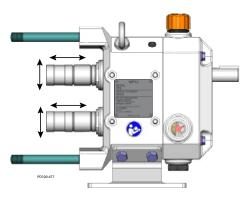
Figure 29 - Bearing Deflection Check
