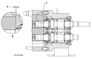
Figure 57 - Rotor to Body Clearance
