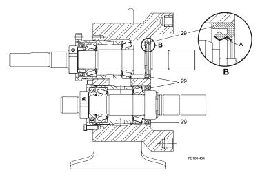
Figure 48 - Apply Bearing Grease
