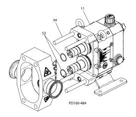
Figure 33 - Pump Body Removal
