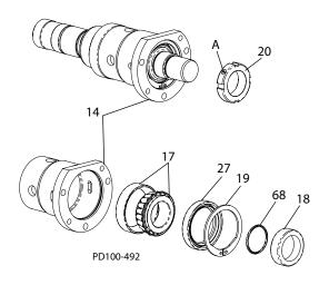
Figure 42 - Remove Bearings
