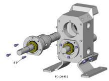
Figure 49 - Secure with Cap Screw
