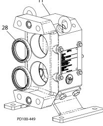
Install new front bearing seals (Figure 44, item 28) into the gear case (item 11) with the primary lip facing toward the inside of the gear case. The seals should be flush with the face of gear case.
