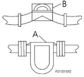
Figure 16 - Inline Strainers and Traps
