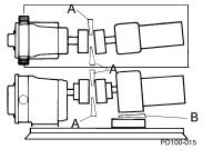
Figure 19 - Check Angular Alignment
