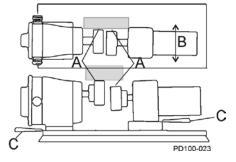
Figure 20 - Check Parallel Alignment
