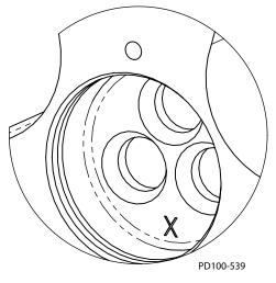
Figure 31 - Counterbore Detail
