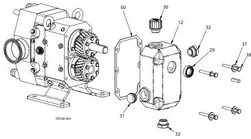
Figure 65 - Gear Cover Installation
