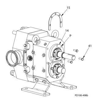
Figure 58 - Install Shims
