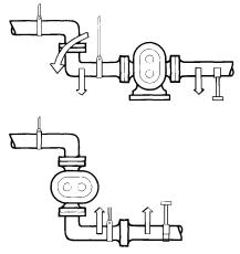
To minimize forces exerted on the pump, support all piping to the pump independently with hangers or pedestals. Such forces can cause misalignment of the pump parts and lead to excessive wear of rotors, bearings, and shafts. Figure 8 shows typical supporting methods used to independently support each pipe, reducing the weight effect of piping and fluid on the pump.
