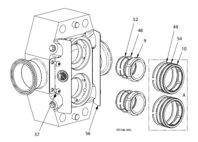
Figure 53 - Shaft Seal Installation
