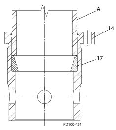
Figure 46 - Press Rear Bearing Cup
