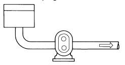
Install the pump below the supply liquid level to reduce the air in the system by flooded suction (Figure 10).
