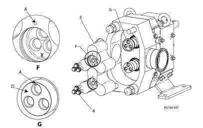
Figure 56 - Rotor Installation
