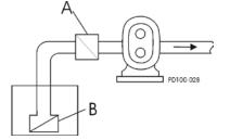
Figure 12 - Inlet Check Valve
