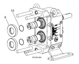
Figure 52 - Shaft Seal Installation
