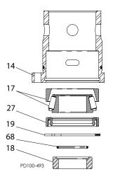
Figure 43 - Press Shaft Free of Rear Bearing
