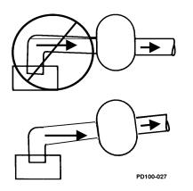
If the pump is installed above the supply liquid level, the piping on inlet side must slope up toward the pump, preventing air pockets in the pipes (Figure 11).
