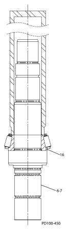
Figure 45 - Press Bearing Cone onto Shaft
