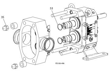
Figure 54 - Body Installation
