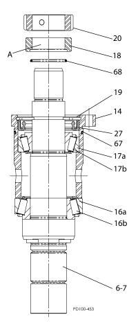
Figure 47 - Bearing Assembly
