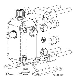
Figure 37 - Remove Oil Drain Plug
