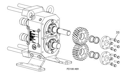
Figure 39 - Remove Gear and Locking Assembly
