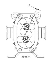
Figure 63 - Rotor Clearance
