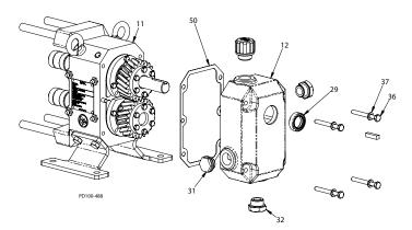
Figure 36 - Remove Gear Case Cover
