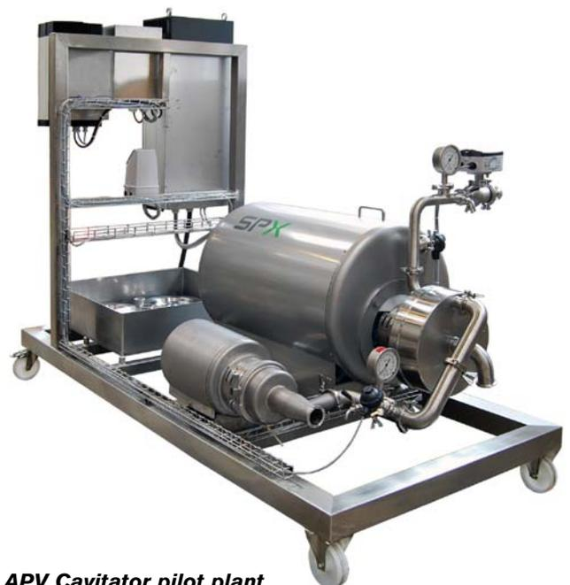
**APV Cavitator pilot plant
