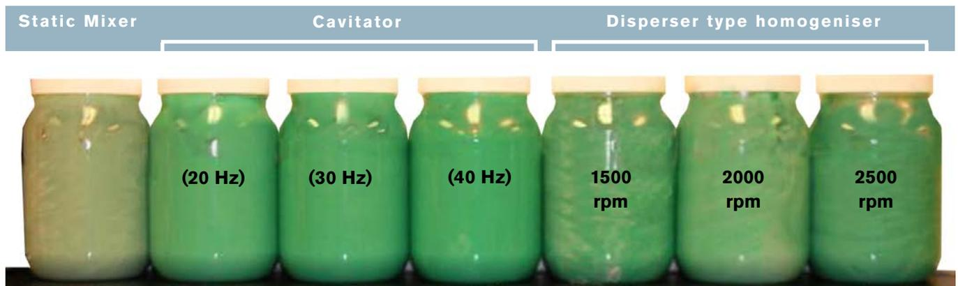
APV Cavitator in comparison with static mixer and homogenizer. Mixing pigment and other post additional ingredients with high viscous base cream liquids.
