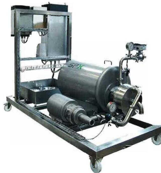
At the heart of the new Cavitator device is a specialised rotor, which is manufactured with equidistant cavities. When the rotor spins, it generates hydrodynamic cavitation within these cavities. Because the cavitation is controlled, there is none of the traditional damage from this process to either the rotor surface or its metal housing (photo: SPX)
