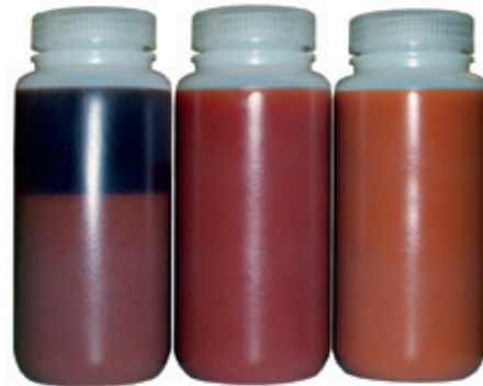
The photo shows the same pre-mix before emulsification, and at two different rotor speeds resulting in different colour due to oil droplet size
