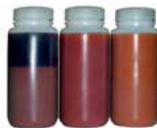
The photo shows the same pre-mix before emulsification, at two different rotor speeds resulting in different color due to oil droplet size
