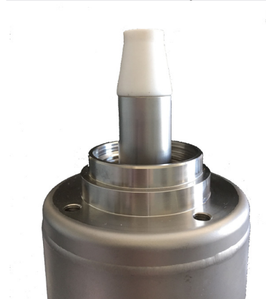
Assembly tool for actuator screw (H338580)
