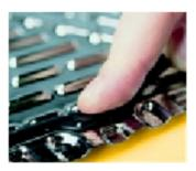
Figure 47: Attachment of EasyClip gaskets
