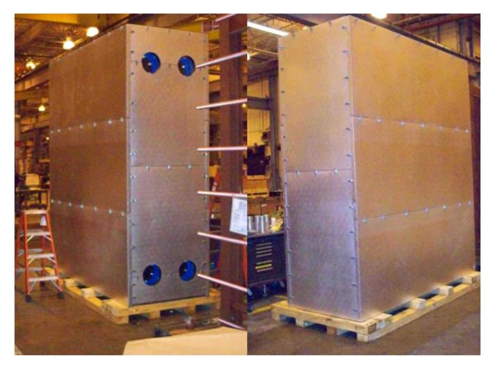
Figure 56: Insulation Jacket
