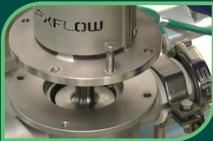
Figure 2. Jack Screw used to facilitate valve disassembly during maintenance
