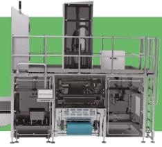
Meeting the latest standards for operator safety and food hygiene, the butter bulk packer offers an efficient solution for fully automatic packaging of butter into carton sizes from 10 kg to 25 kg. Ideal for use with various butter products, the machine can also handle other types of crystallized fats, including vegetable fat and dairy blends.
