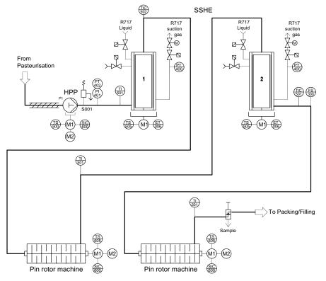
Figure 3: Process for recombined butter by SSHE technology
