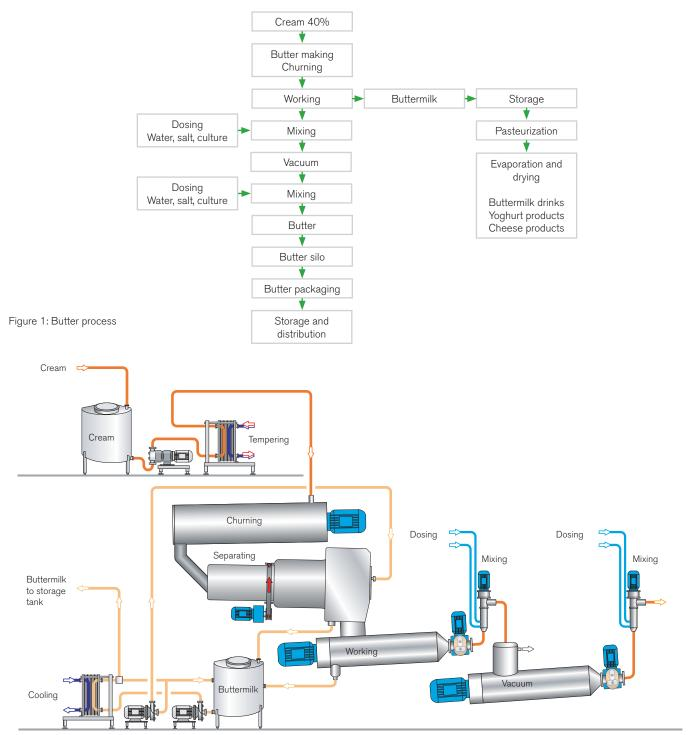
Figure 2: Principle of a butter machine
