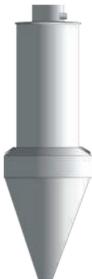
The optimal choice for drying of whey protein concentrate and isolate is SPX FLOW's Anhydro Tall Form spray dryer, designed with a cylinder and a cone with bustle, to deliver optimal conditions for gentle drying of proteins. The air distributor is customized for optimal performance and the dryer is equipped with an external fluid bed. The dryer is designed with the latest safety equipment to comply with legal and industrial standards.
