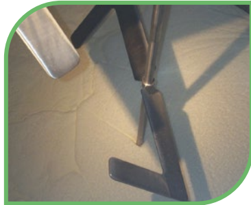
Zeta impellers before re-starting mixer operation, after yogurt fermentation.
