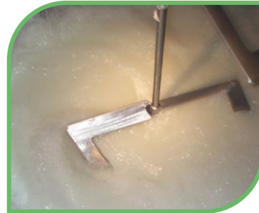
Zeta impellers mixing yogurt in the vessel to a homogeneous state, before further processing.
