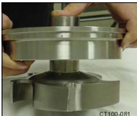
Figure 25 - Moving Rotary Seal Up the Shaft
