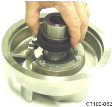
Figure 26 - Push Rotary Seal Down
