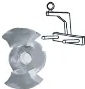
USE ROTOR REMOVAL TOOL TO REMOVE ROTORS
