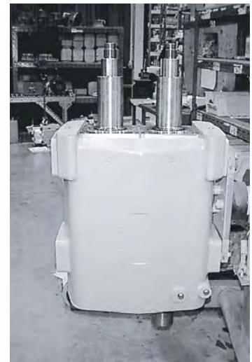
SHAFT ASSEMBLY REMOVAL WITH TOOL
