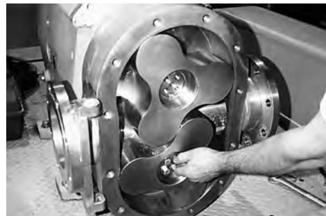
3. REMOVE ROTOR RETAINING BOLTS
