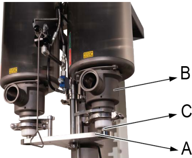
Figure 50 - Location Of Dual Cylinder Foot and Position Holding Arm
