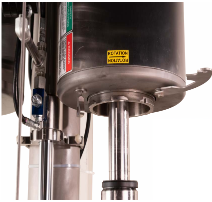
Figure 79 - Exposing Top Mechanical Seal
