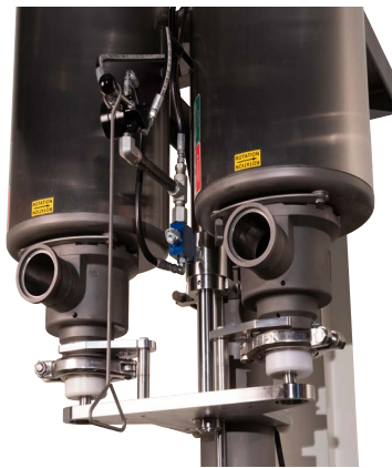
Figure 24 Location of Dual Cylinder Foot and Position Holding Arm
