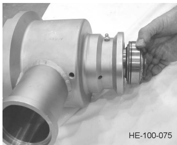
Figure 44 - Install Head Shaft Bearing
