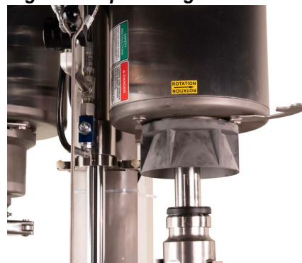
Figure 30 Install Blade Alignment Cone
