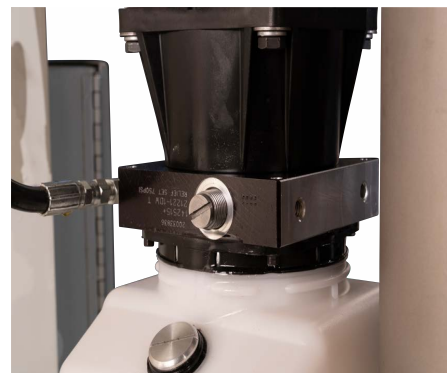
Figure 22 Pressure Adjustment Screw- cap removed
