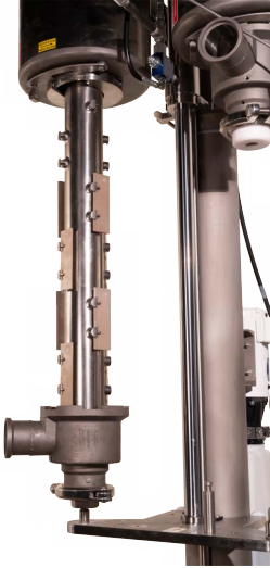
Figure 26 Lower the mutator shaft
