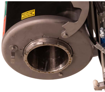
Figure 57 - Remove Front Jacket Cover Bolts
