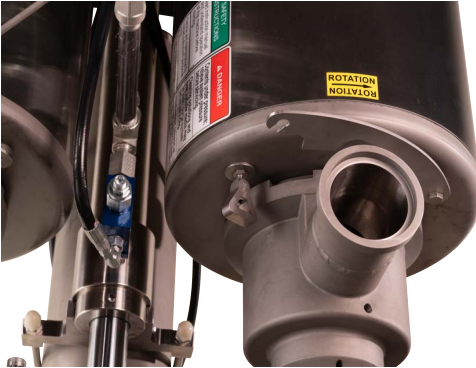
Figure 56 Close Locking Latch
