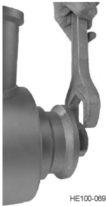
Figure 45 - Installation of Shaft Locknut
