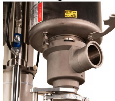
Figure 25 Disengaging Locking Latch and Opposite Drive Head
