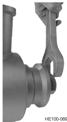
Figure 35 - Removal of Shaft Locknut
