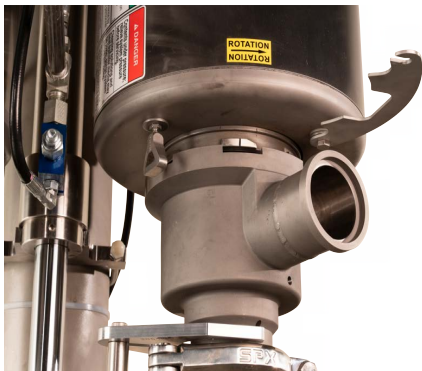
Figure 51 - Disengaging Locking Latch and Opposite Drive Head
