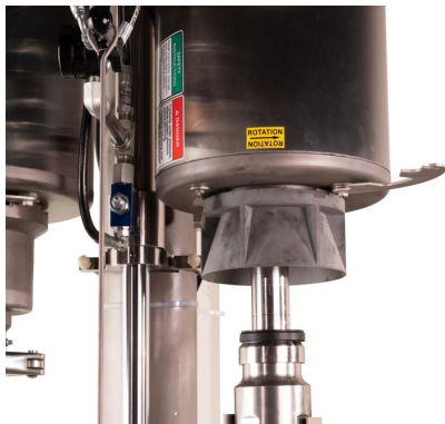
Figure 54 - Install Blade Alignment Cone
