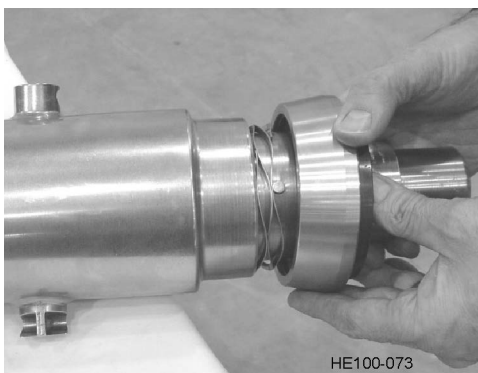
Figure 41 - Mechanical Seal Installation
