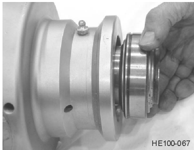
Figure 31 - Lubrication Ring Orientation
