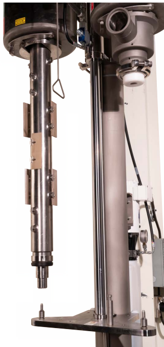
Figure 83 - Shaft With Head Removed
