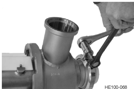
Figure 34 - Removal of Hinged Clamp
