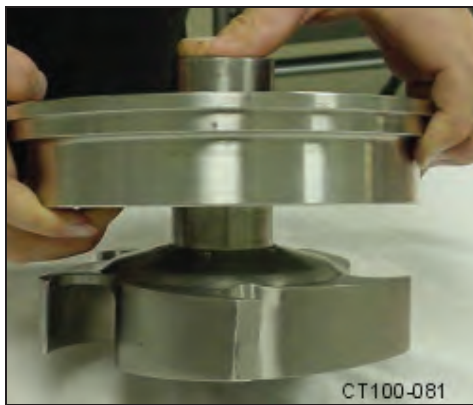
Figure 26 - Moving the Rotary Seal up the Shaft
