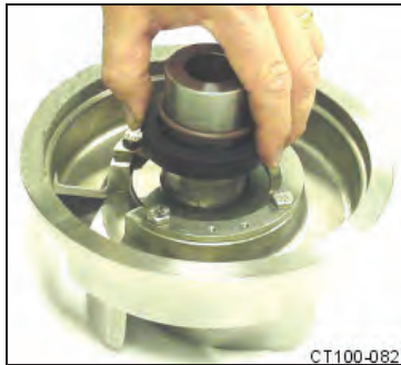
Figure 40 - Push Rotary Seal Down Until o-ring is Released.
