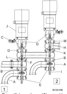
Figure 15: Inspection and Disassembly Steps
