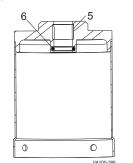
Figure 20: Remove O-ring and Bearing
