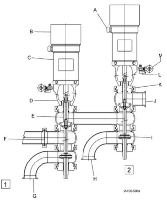
Figure 1: Flow Diversion Valve Nomenclature
