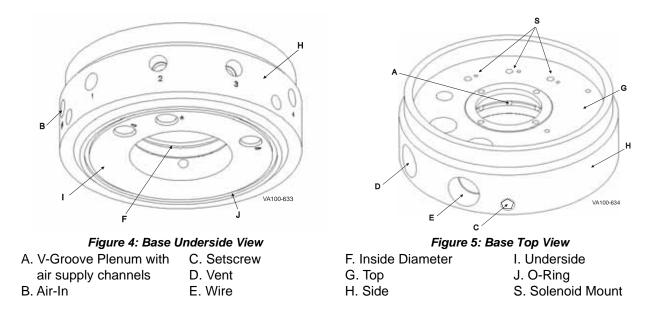
Compressed air is routed through the base from **Air-In** (item B) to a V-groove air-plenum (item A) in the inside diameter (item F). Supply channels from the plenum feed each of three (3) threaded solenoid mounts (item S) on top. An energized solenoid passes air to the non-threaded outlet hole, feeding the corresponding side (item H) and underside (item I) air ports.
