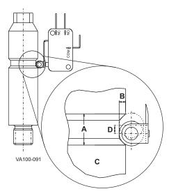
Figure 13: Detail of the Micro Switch Position for Divert Mode
