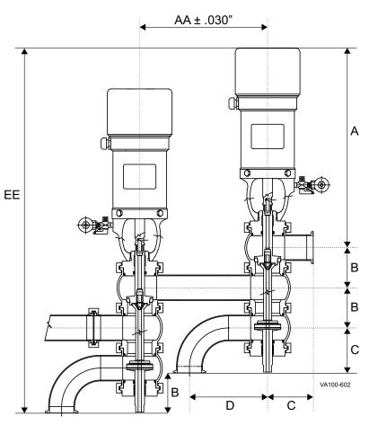
Figure 3: Valve Dimensions
