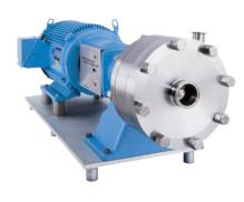
SPX FLOW offers three single stage and one multistage high-pressure 200 Series centrifugal pump models. Designed for use in membrane filtration systems (reverse osmosis and ultra filtration), they can accommodate high system pressure inlet conditions to 1000 psi (69 bar) producing a smooth, pulse-free high discharge pressure for reduced membrane wear and increased product quality.
