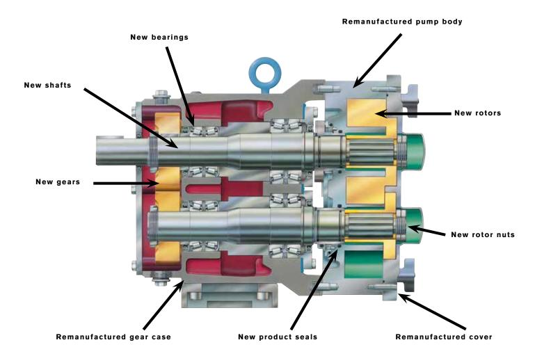
The remanufacture program provides the customer with **standard** oversized tolerances. This option maximizes interchangeability of parts within the customer's operation.
