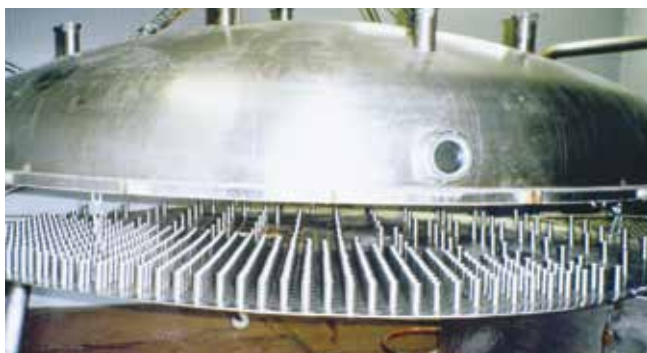
Liquid distributor of MVR evaporator
