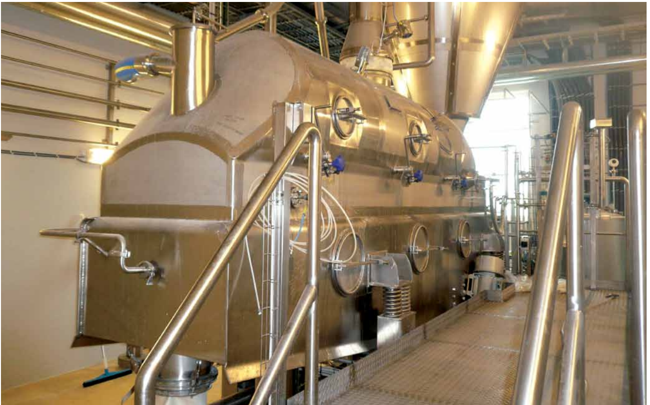
Anhydro chamber with integrated and external fluid bed for drying
