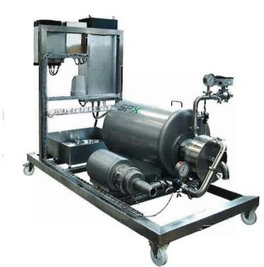
At the heart of the new Cavitator device is a specialised rotor, which is manufactured with equidistant cavities. When the rotor spins, it generates hydrodynamic cavitation within these cavities. Because the cavitation is controlled, there is none of the traditional damage from this process to either the rotor surface or its metal housing (photo: SPX)
