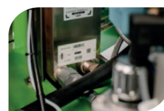
External oil cooling with automatic temperature control Reduced cooling water consumption. Stable operation through increased cooling capacity and better controls
