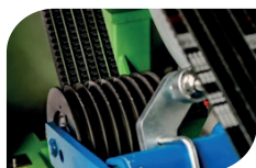
Automatic Belt Tensioner Reduced maintenance – increased belt lifetime and longer service intervals
