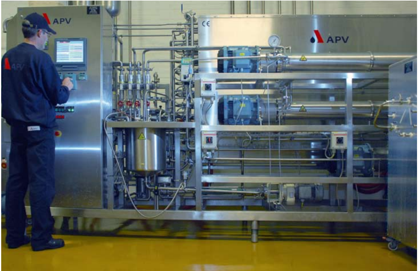
APV LeanCreme Pilot Plant for microparticulation of whey
