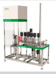
**Principle:** Frozen or lyophilized starters are introduced manually in a dosing vat system (DVS) before being flushed to the fermentation or storage tank by milk coming from the pasteuriser.
