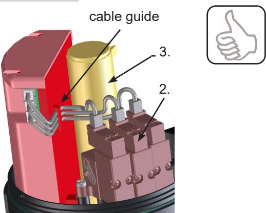
The cable/s by means of which the solenoid valves are connected with the electronic module must be guided through the cable guide at the rear side of the electronic module (fig. 3.2.1).
