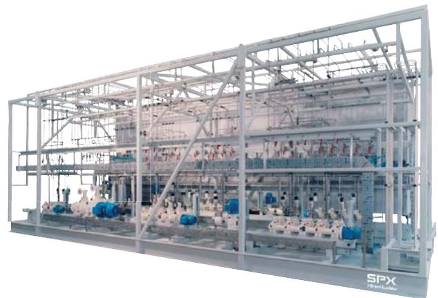
**Compact two-tier package designed to provide storage and injection of wax inhibitor and scale inhibitor, on a bunded base frame, within a very tight space constraint, on an existing platform**
