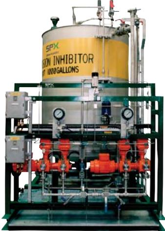
**Methanol injection package incorporating Bran+Luebbe double diaphragm, double-acting pumps for offshore platform**
