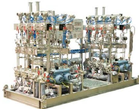
**Chemical dosing skid for sulphate removal module on Floating Production Unit (FPU)**
