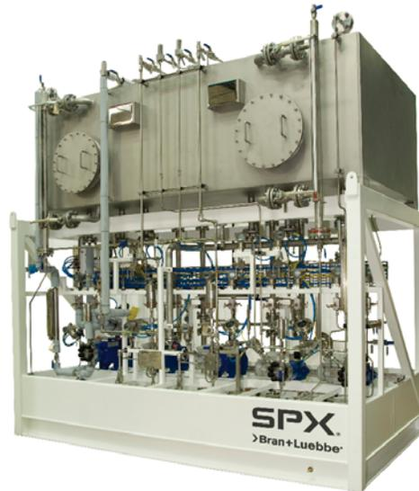
**Glycol and corrosion inhibitor package for onshore use at a gas storage plant. Package incorporates a double wall tank with leak detection system, IBC laydown area, injection pumps system, and rain shelter**
