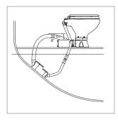
Toilet mounted above the waterline and discharging overboard.
