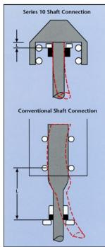
Distance between seal face and rigid support (L) is shorter in Series 10 design compared to conventional design, minimizing shaft deflection at seal face.
