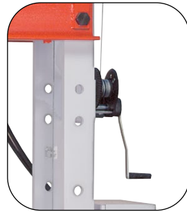
Winch provides easy positioning of press bed
