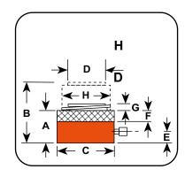
**NOTICE:** When selecting a hydraulic cylinder(s) capacity and stroke, Power Team recommends that you size to 80% of the maximum rated capacity and stroke for the application - known as the "80% Rule". This will ensure additional safety factor and extend the product performance over time.
