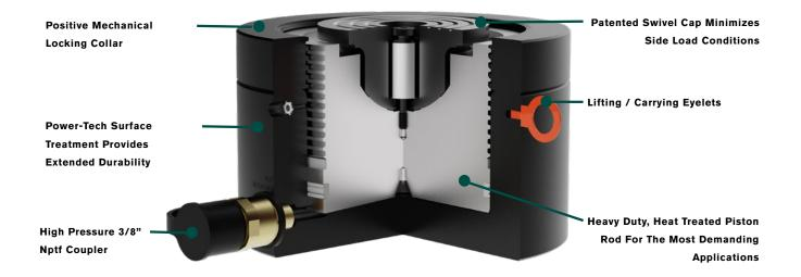
**NOTICE:** When selecting a hydraulic cylinder(s) capacity and stroke, Power Team recommends that you size to 80% of the maximum rated capacity and stroke for the application - known as the "80% Rule". This will ensure additional safety factor and extend the product performance over time.
