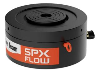
Power Team's RGP Series of construction pancake cylinders are ideal for applications that require lifting in tight or confined spaces, such as bridge bearings on end caps or piers. The RGP Series is available with lifting capacities from 55 – 565 Tons (60,8 – 512,6 Tonne).
