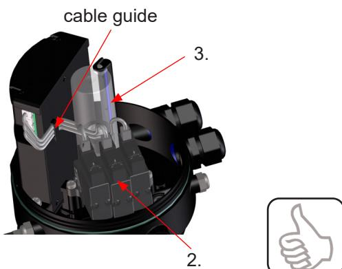
The cable/s by means of which the solenoid valves are connected with the electronic module must be guided through the cable guide at the rear side of the electronic module. (fig. 3.2.1).
