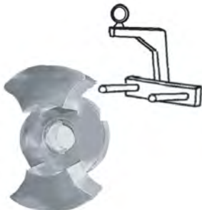
USE ROTOR REMOVAL TOOL TO REMOVE ROTORS
