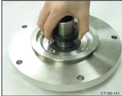
Figure 15 - Move Rotary Seal Up Shaft
