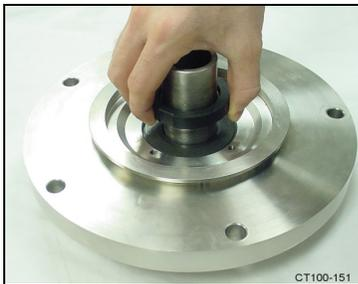
Figure 20 - Move Rotary Seal Up Shaft
