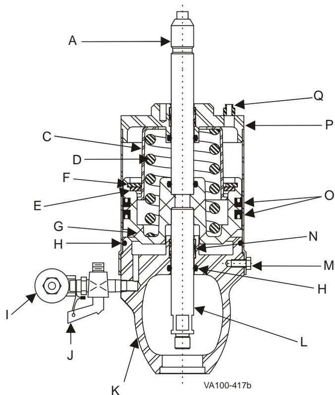
**Figure 2: Actuator Components**
