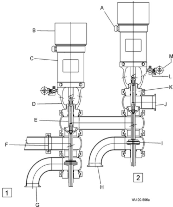
**Figure 1: Flow Diversion Valve Nomenclature****Callouts for Figure 2:**
