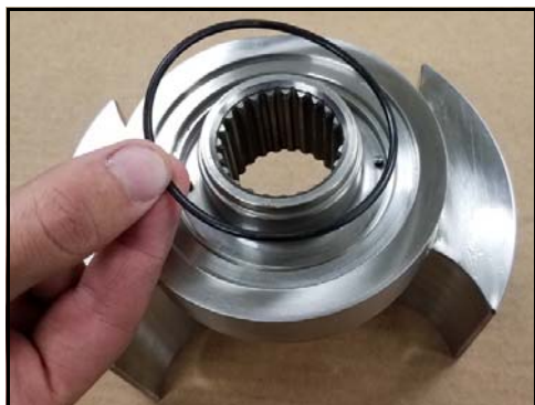
Figur 169 - Montér muffens forreste O-ring
