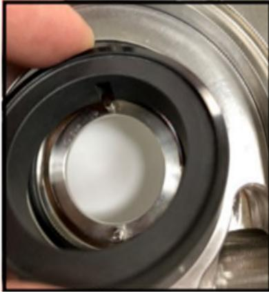
**Figure 70** Installation de garniture fixe
