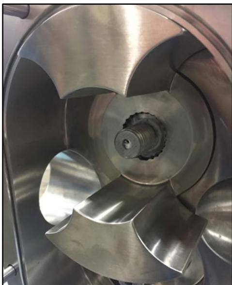
**Figure 256 - Rotor installé**
