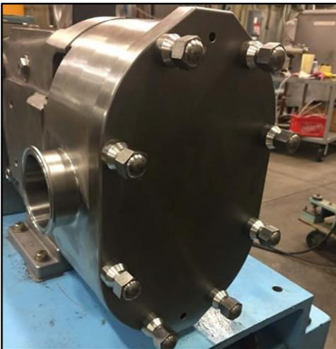
**Figure 266 - Couvercle installé**
