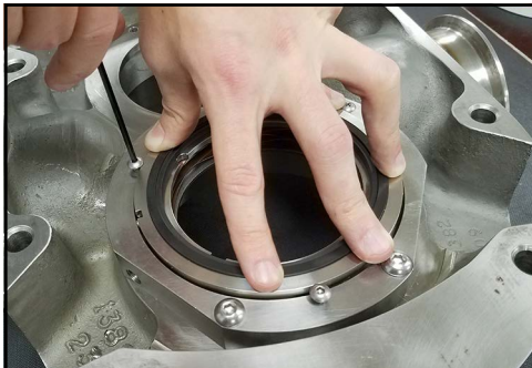
Figure 195 - Install seal retaining bolts
