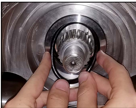
Figure 246 - Install seal O-ring
