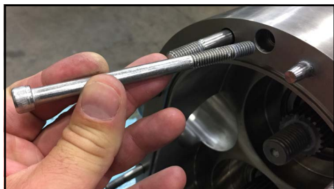
Figure 225 - Remove body retaining screws
