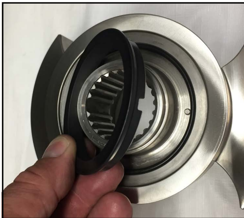
Figure 215 - Install rotary seal
