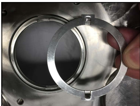
Figure 156 - Remove drive ring
