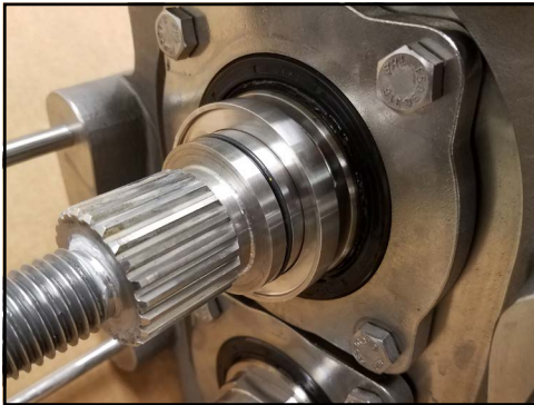
Figure 241 - Seal seat installed
