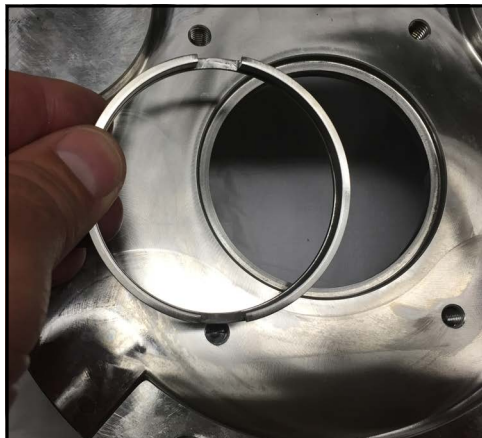
Figure 127 - Remove shaft ring
