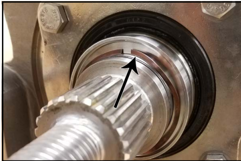
Figure 230 - Remove wave spring
