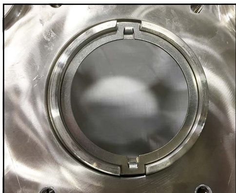
Figure 162 - Drive ring installed
