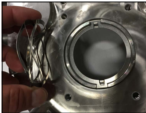
Figure 133 - Install wave spring
