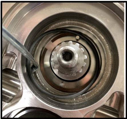
Figure 55 Remove stationary seal O-ring
