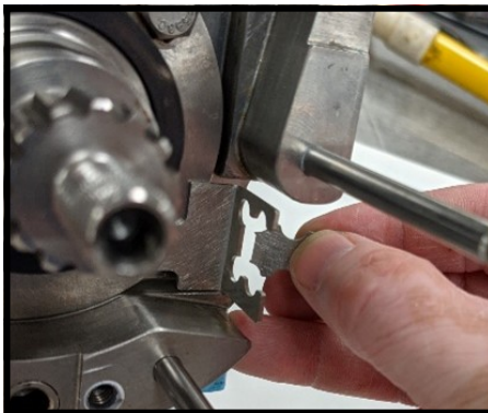
Figure 106 Break tab off finger guard
