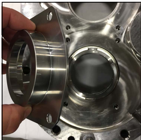
Figure 135 - Install seal housing
