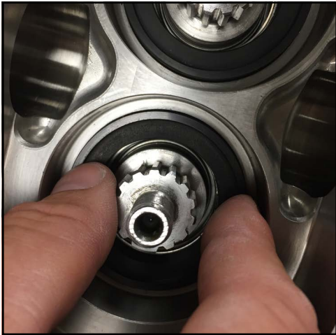
Figure 211 - Push on stationary seal
