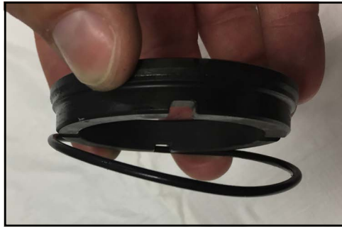
Figure 119 - Remove stationary seal O-ring
