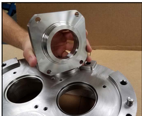
Figure 234 - Line up bolt holes
