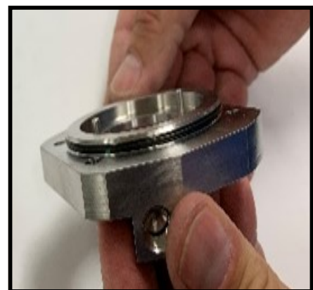
Figure 92 Install the seal housing O-ring
