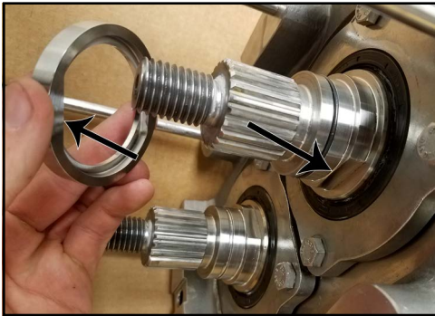
Figure 240 - Install seal seat
