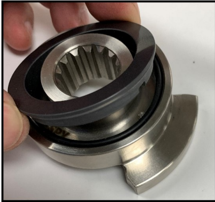
Figure 52 Remove rotary seal
