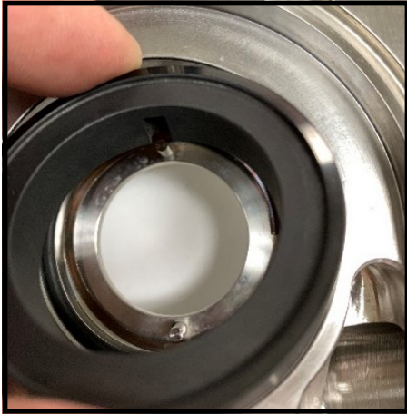
Figure 70 Install stationary seal
