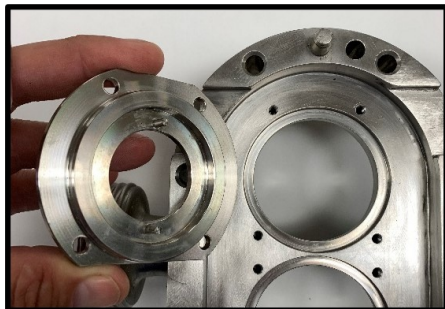
Figure 60 Remove seal housing
