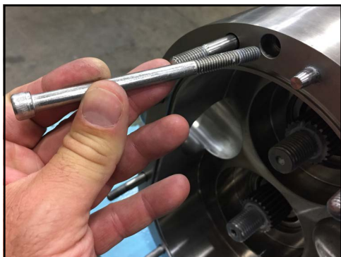
Figure 67 - Install body retaining screws
