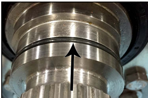
Figure 147 - Adjusting ring O-ring
