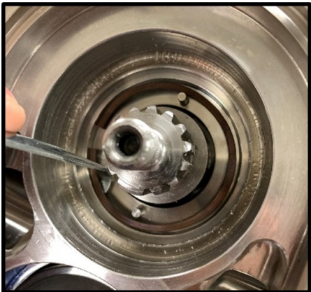
Figure 56 Remove stationary seal wave spring
