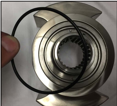
Figure 213 - Install seal O-ring
