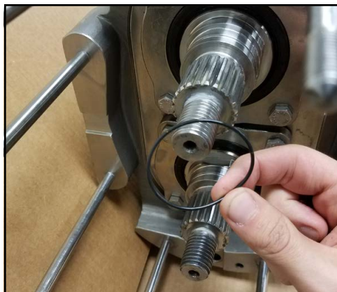
Figure 238 - Lubricate and install O-ring
