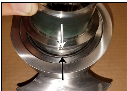
Figure 249 - Line up notch and pin
