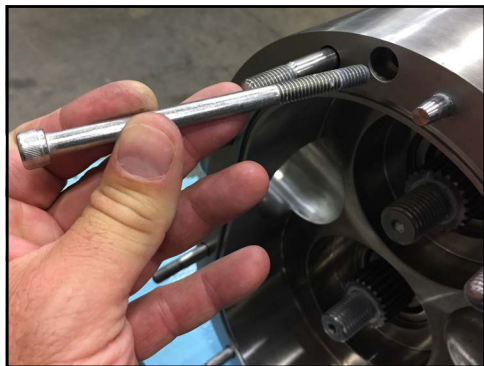
Figure 207 - Install body retaining screws
