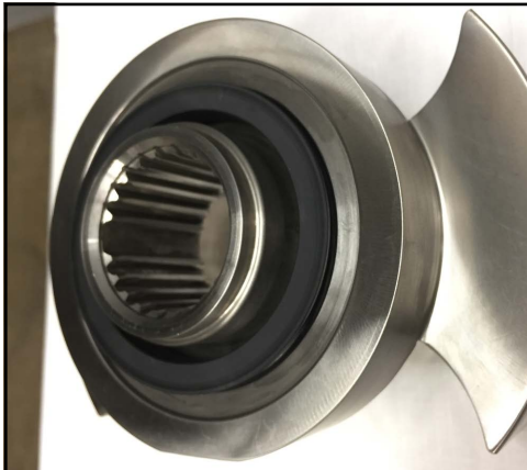
Figure 216 - Rotary seal installed
