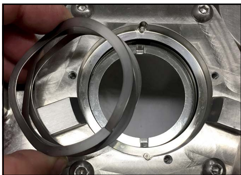
Figure 170 - Install wave spring
