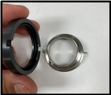
Figure 82 Remove flush side rotary seal and O-ring
