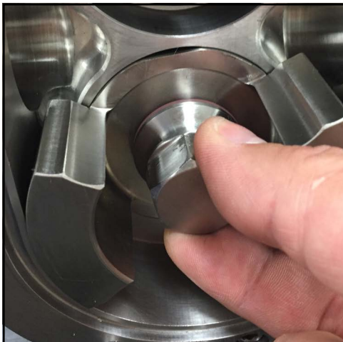
Figure 259 - Install rotor nut
