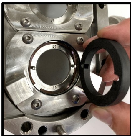
Figure 85 Remove stationary seal
