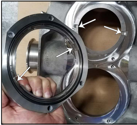
Figure 188 - Seal housing O-ring installed
