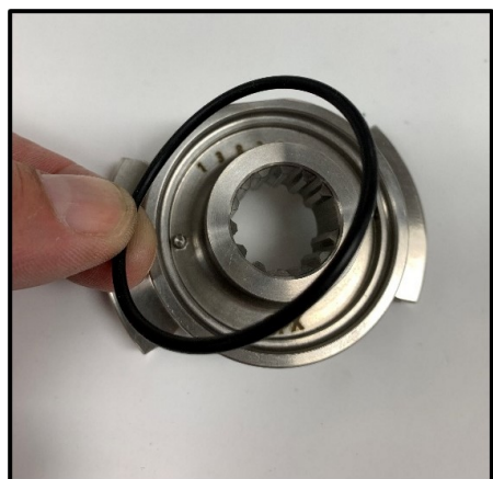
Figure 114 Install seal O-ring
