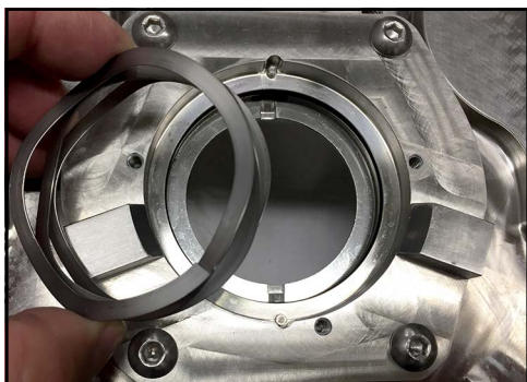
Figure 150 - Remove wave spring
