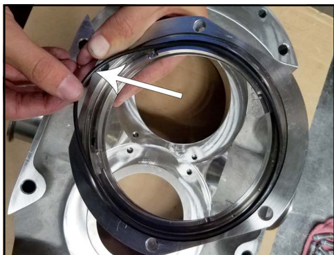
Figure 155 - Remove seal housing O-ring
