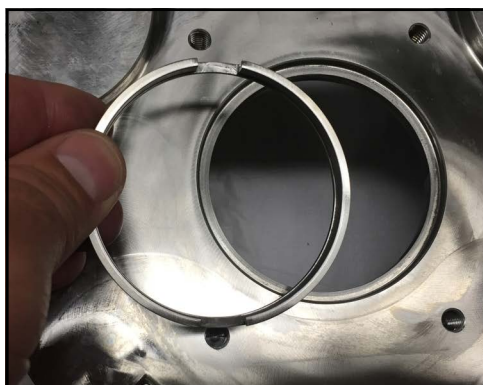
Figure 129 - Install shaft ring
