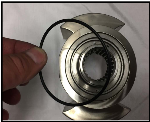
Figure 117 - Remove seal O-ring
