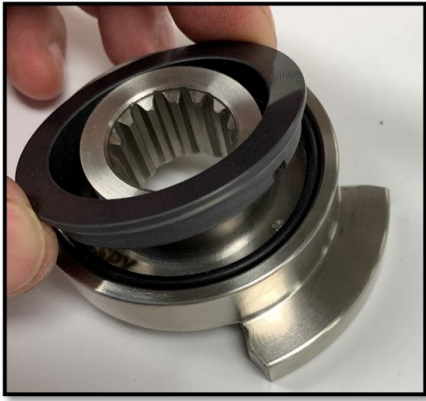
Figure 115 Install rotary seal
