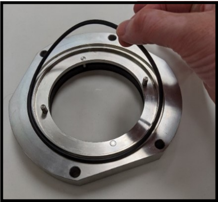
Figure 93 Install the seal housing O-ring
