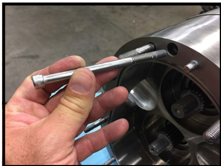
Figure 79 Remove body retaining screws
