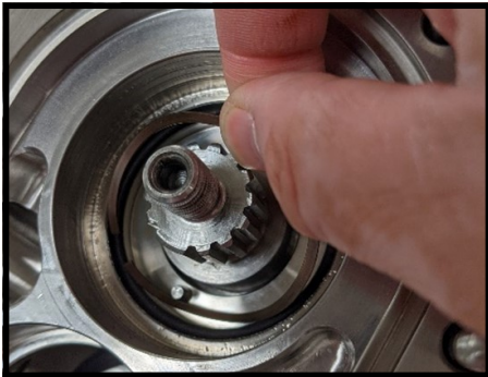
Figure 111 Install stationary wave spring
