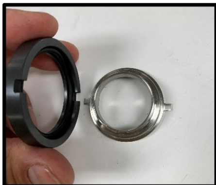
Figure 104 Install flush side rotary seal
