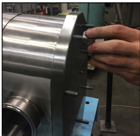
Figure 265 - Install cover nuts
