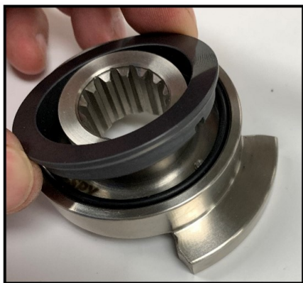
Figure 51 Install rotary seal
