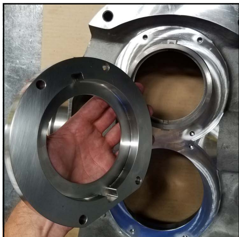
Figure 141 - Install seal housing
