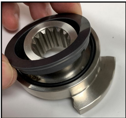
Figure 74 Remove rotary seal
