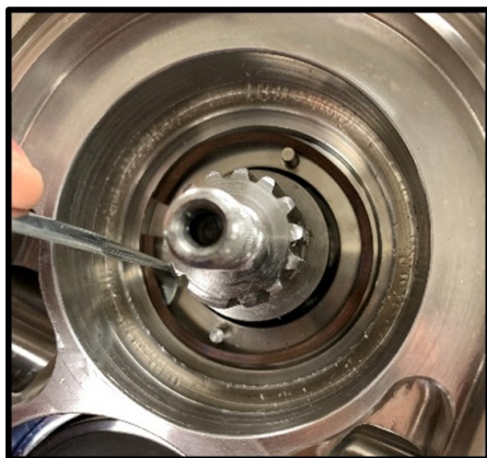
Figure 78 Remove stationary seal wave spring
