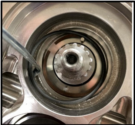
Figure 44 Remove stationary seal O-ring
