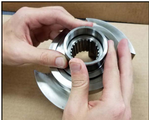
Figure 250 - Press sleeve into place
