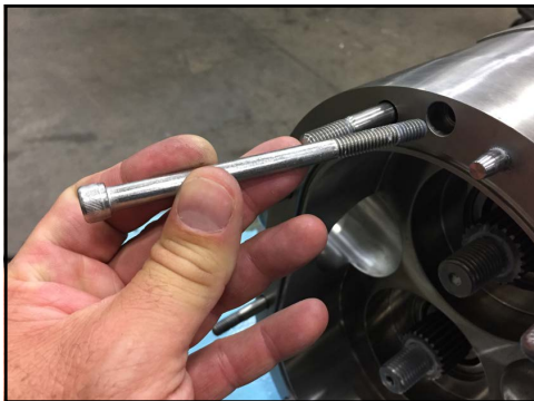
Figure 245 - Install body retaining screws
