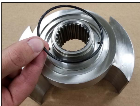
Figure 247 - Install sleeve front O-ring
