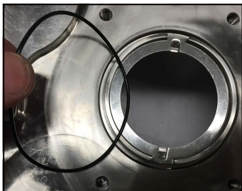
Figure 163 - Install seal housing O-ring
