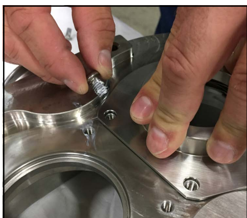
Figure 136 - Install seal housing bolts
