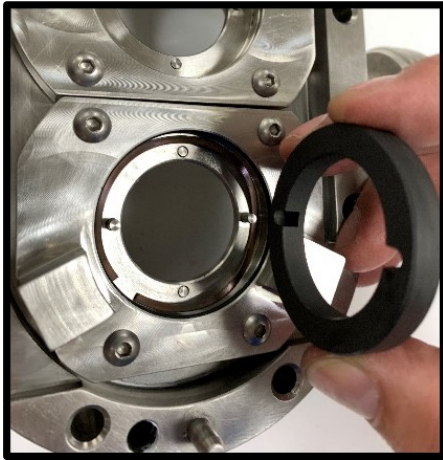
Figure 99 Install stationary seal
