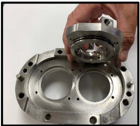
Figure 94 Install seal housing
