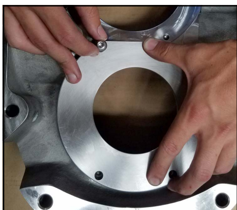
Figure 142 - Install seal housing bolts
