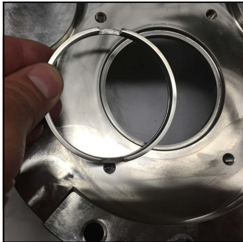
Figure 159 - Install shaft ring
