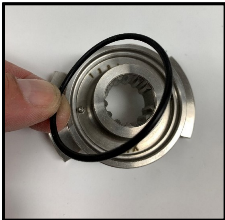
Figure 75 Remove seal O-ring
