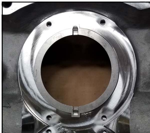
Figure 139 - Drive ring installed
