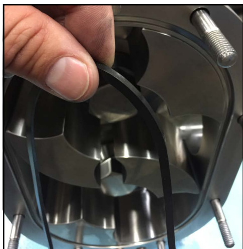
Figure 37 - Remove cover gasket
