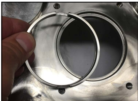
Figure 157 - Remove shaft ring
