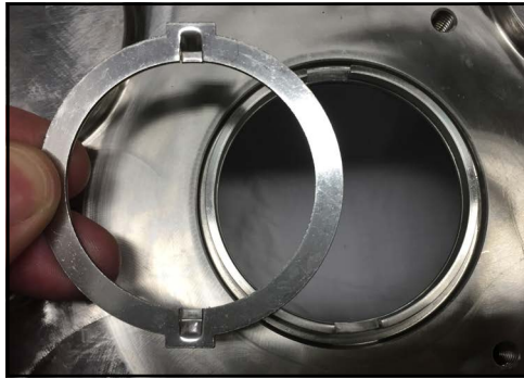
Figure 131 - Install drive ring
