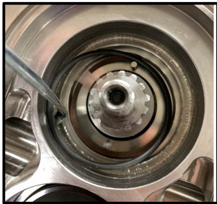
Figure 77 Remove stationary seal O-ring
