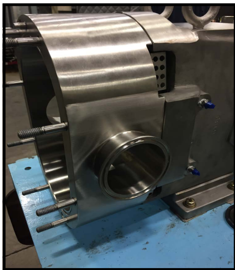
Figure 108 - Pump body installed
