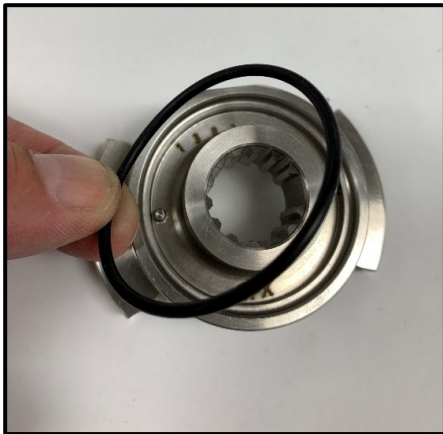
Figure 42 Remove seal O-ring
