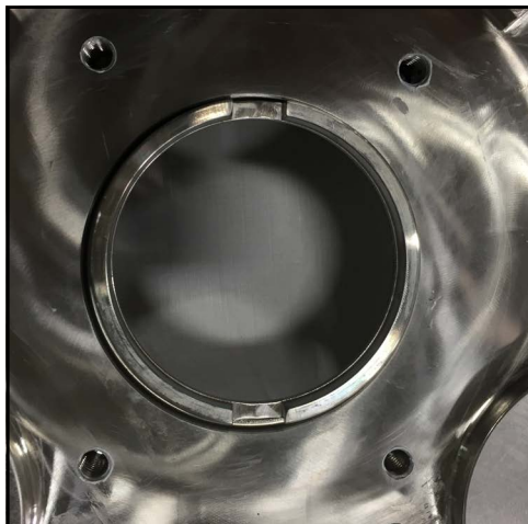
Figure 160 - Shaft ring installed
