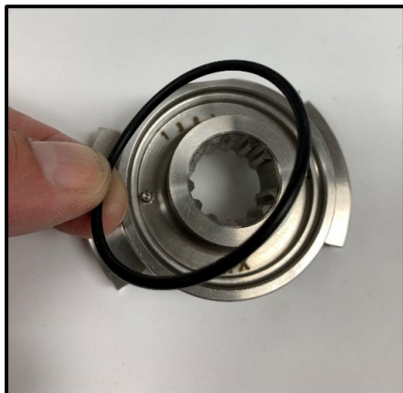
Figure 72 Install seal O-ring
