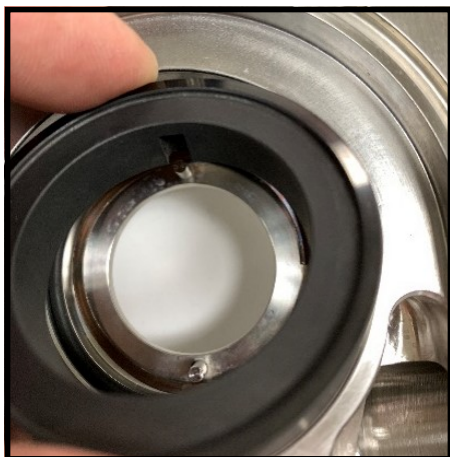
Figure 112 Install stationary seal
