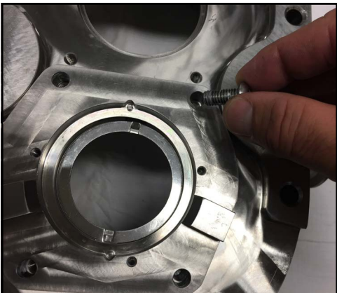
Figure 166 - Seal housing bolts
