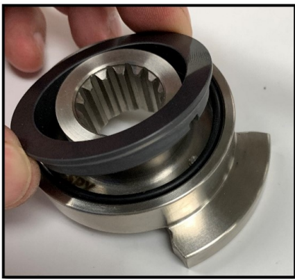
Figure 73 Install rotary seal
