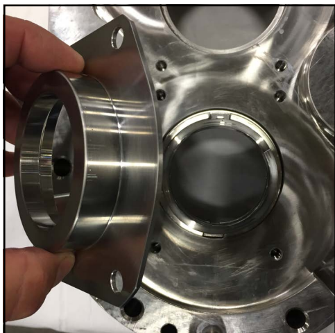
Figure 123 - Remove seal housing
