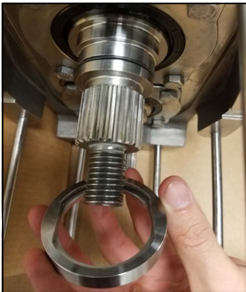
Figure 231 - Remove seal seat
