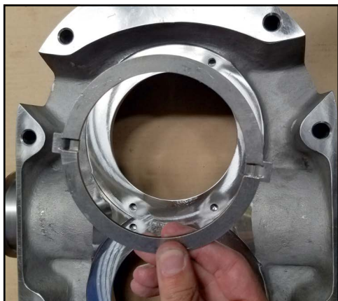
Figure 185 - Install drive ring
