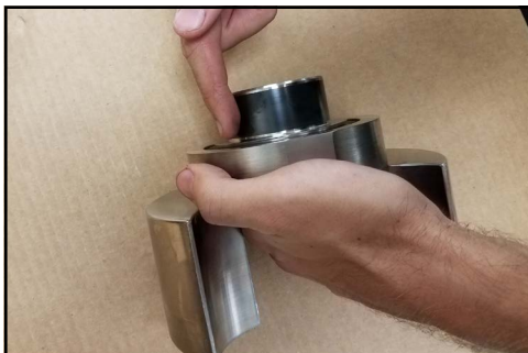
Figure 252 - Lubricate seal sleeve
