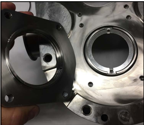
Figure 165 - Install seal housing
