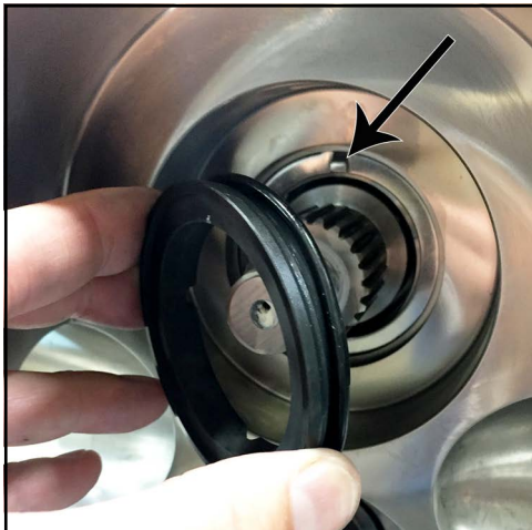
Figure 210 - Install stationary seal
