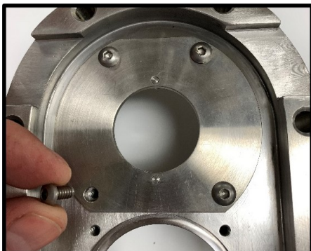
Figure 63 Install seal housing bolts
