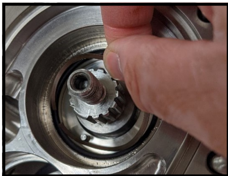
Figure 69 Install stationary wave spring
