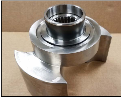
Figure 251 - Seal sleeve installed
