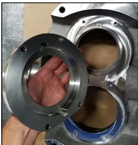
Figure 124 - Remove seal housing
