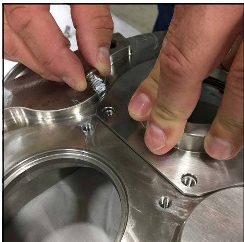
Figure 122 - Remove seal housing bolts
