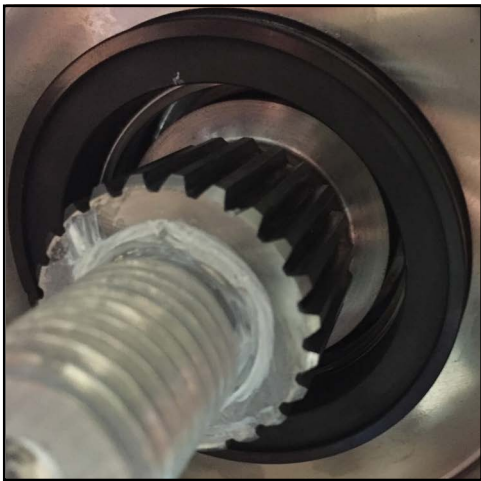
Figure 212 - Stationary seal installed
