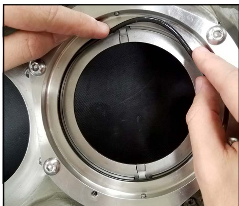
Figure 191 - Install seal O-ring
