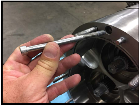
Figure 109 - Install body retaining screws
