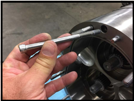
Figure 57 Remove body retaining screws
