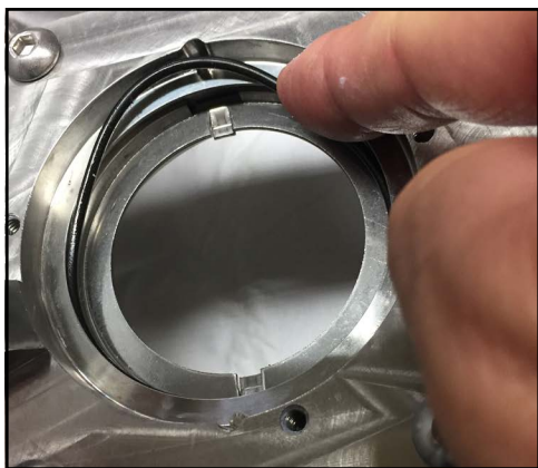
Figure 168 - Install seal O-ring
