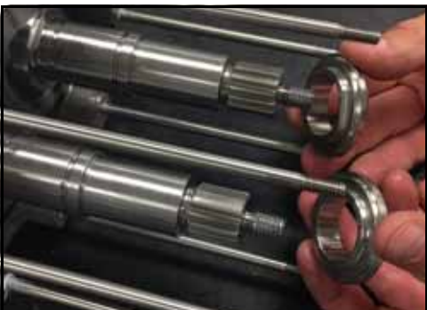
Figure 215 – Installation des bouchons de garniture
