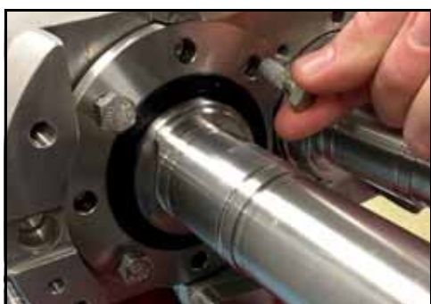
Figure 200 – Installation des rotors
