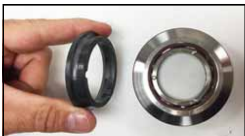
Figure 73 – Lubrification et installation de la garniture
