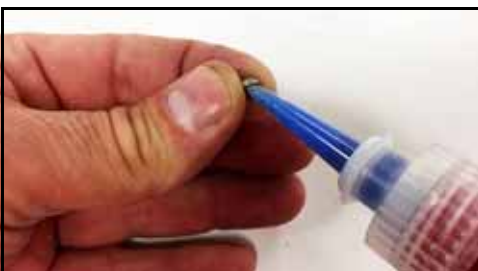
Figure 231 – Application de colle Loctite®
