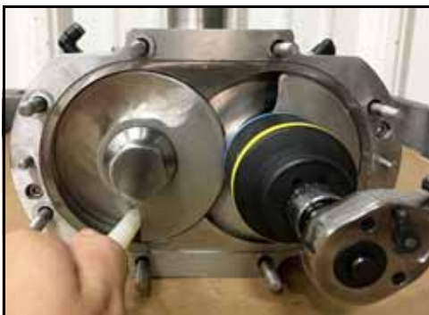
Figure 121 – Insertion de la cale
