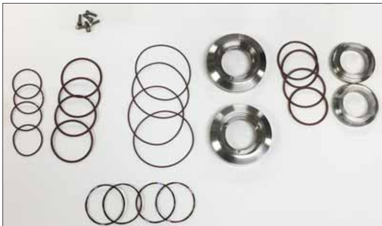
Figure 63 – Composants de la garniture
