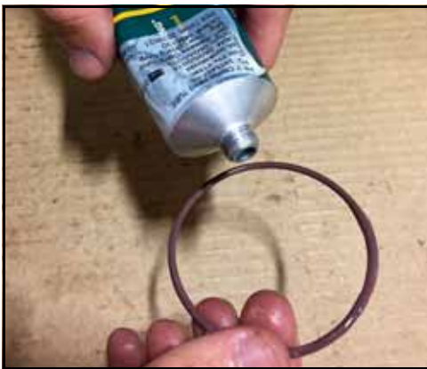
Figure 83 – Lubrification des joints toriques
