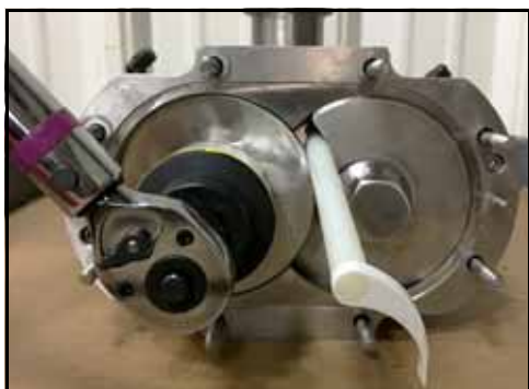
Figure 123 – Insertion du goujon
