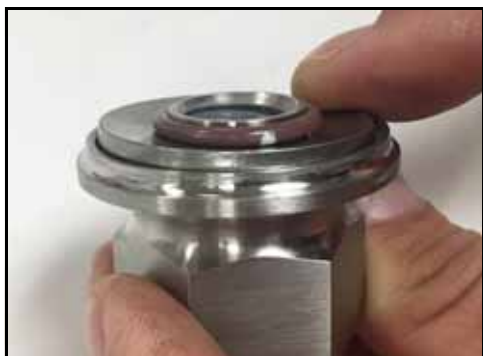
Figure 115 – Rondelle Belleville installée
