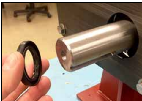
Figure 238 – Installation du joint d’huile
