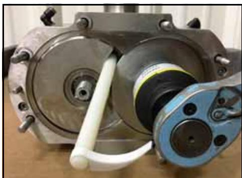
Figure 34 – Insertion du goujon
