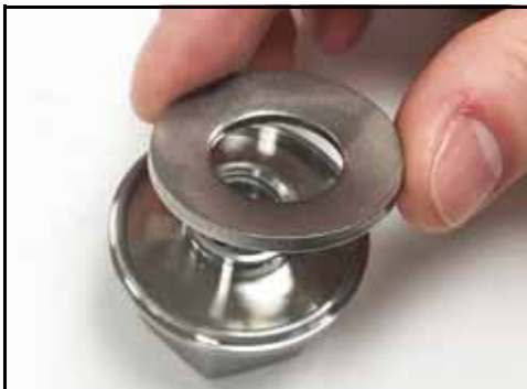
Figure 113 – Installation de la rondelle Belleville
