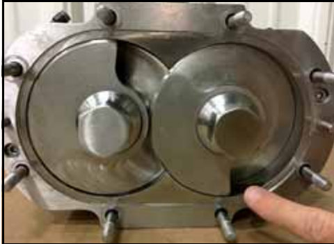
Figure 31 – Rotation des rotors
