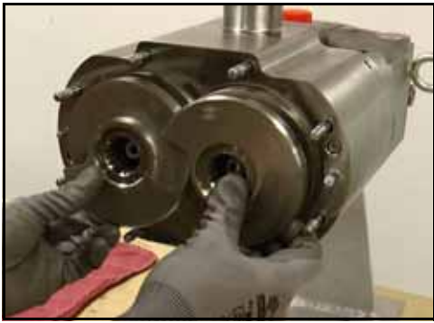
Figure 109 – Installation des rotors
