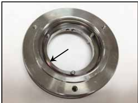
Figure 71 – Ressort ondulé de la garniture installé
