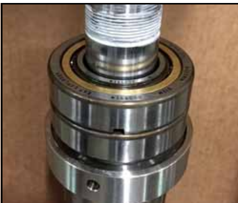
Figure 173 – Second roulement installé
