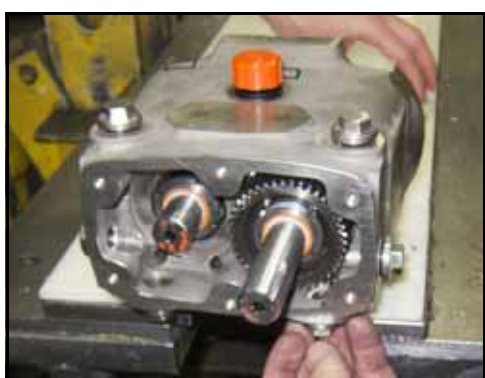
Figure 209 – Installation des bouchons
