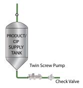
Our twin screw pump is both process and CIP and SIP capable, allowing you to reduce the number of pumps, valves and controls in your process saving capital and running costs.
