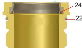
fig. 24: Assembly tool for actuator screw (H338580)
