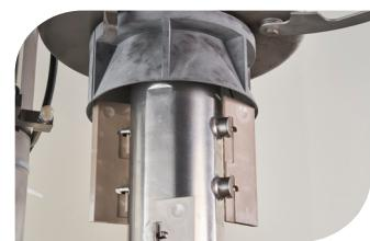
**Blade alignment tools** - new two piece wide-angled lightweight blade alignment cone folds the scraper blades inwards during shaft insertion mode
