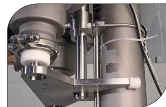
**New dynamic foot assembly for single or dual lift** - Foot is captured by both the guide rod and guide rollers for controlled vertical motion
