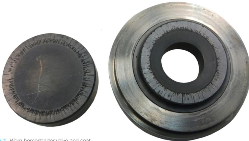
Image 1. Worn homogenizer valve and seat
